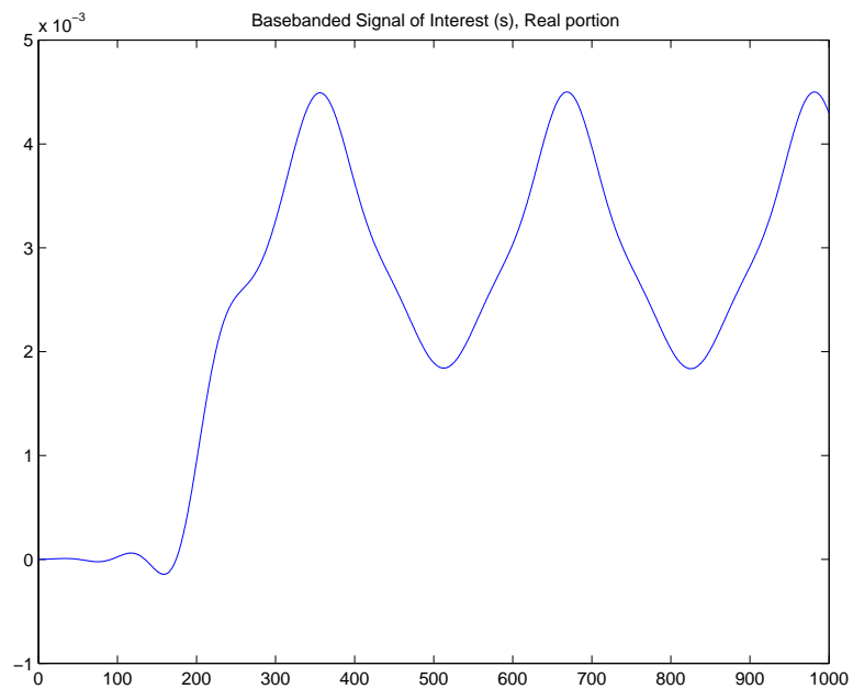
Figure 4.28: Plot of the base-banded version of the signal of interest. This is the envelope of the signal, s , added to the primary channel.
