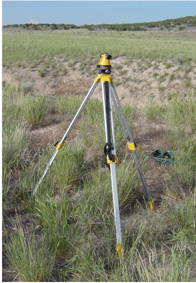
Figure 3.3: Picture of the builders level used to sight the antenna positions.
