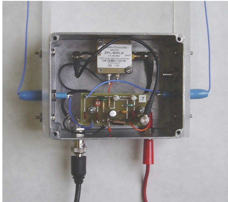
Figure 2.5: RF box. The inputs to the box from the antenna are the connectors on each side. The circuit board at the bottom of the box contains the matching network and current amplifier. At the top of the box is a Mini-Circuits LNA. Coming out the bottom of the box are the signal cable and the power cable which run to the receiver.
